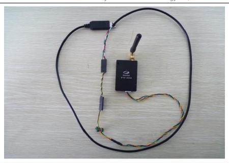
Because the Data Radio via USB-TTL data cable to power on, the Data Radio will immediately into work state when it power on, so the antenna should be installed before the USB-TTL data cable connected to the computer, in order to avoid Data Radio frequency power amplifier circuit part overheat and burn out.
