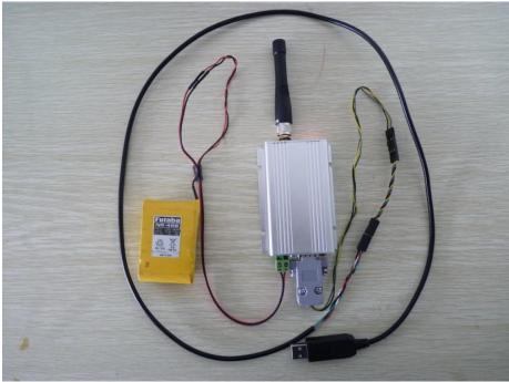
When you power on the Data Radio, the data radio data state LED will flash one time, and power state LED will stay on solid, like the picture below, the LED which near the antenna is data state LED, and the one stay on solid is power state LED:
