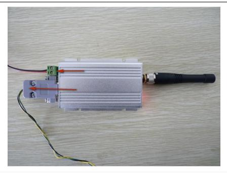
Like FY-602, the Data Radio will immediately into work state when it power on, so the antenna should be installed before power on, in order to avoid Data Radio frequency power amplifier circuit part overheat and burn out.
