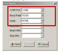
If serial open failed, please check the serial number is correct or not. If the serial number is correct, please re-plugged the USB-TTL data cable. When serial port is open, please click on the 'Search(S)
