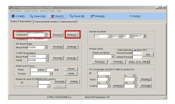
After configuration is "OK" ,please save the parameters to the Data Radio, otherwise the parameters will back to before after power off. Click on the "Write(W)", the software will save the parameters to the data radio, please re-detected again and read the current parameters, if the parameters is the setting parameters, then the parameters have fully configured and saved into the data radio success:
