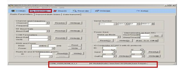
After detected the Data Radio, read the current various parameter values, you can choose "Read(R)" read all parameters, also you can click each item of the "read" readout parameters of this item:
